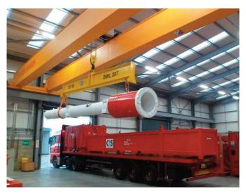
be loaded indoors and with much greater speed and efficiency. Previously this operation was carried out by hiring in a mobile crane, which was not only costly and less efficient, it meant the whole process had to be undertaken outdoors."
