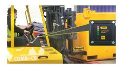
The Combi Safelift anti-overload device detects, alarms and shuts down operation to prevent overloading, without operators
