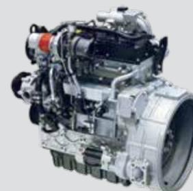
The Doosan G2 Engine meets and exceeds all Euro Stage IIIB (55 kW) and IV (74 kW) emission regulations without a Diesel Particulate Filter (DPF). A Diesel Oxidation Catalyst (DOC) and Selective Catalytic Reduction (SCR) is required for the 74 kW engine. Additional maintenance such as Regeneration or Ash cleaning is not required.
